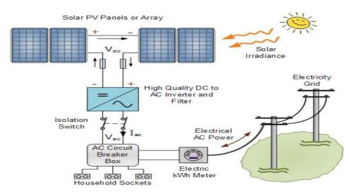
Figure 1.2: Micro Grid connected PV system (Source MNRE 2011)
