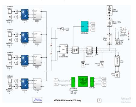
Figure 1.5 Matlab/ Simulink model of 400 kW PV array Micro grid.
